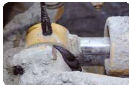
When manually lubricating a bearing, grease is not typically evenly spread inside the bushing and not completely purged
