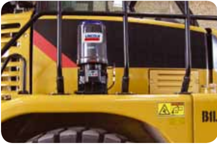
A Datalogger pump safely mounted on the deck level. This pump is connected to a GPS or machine monitoring system that will remotely notify the operator if the system requires service.
